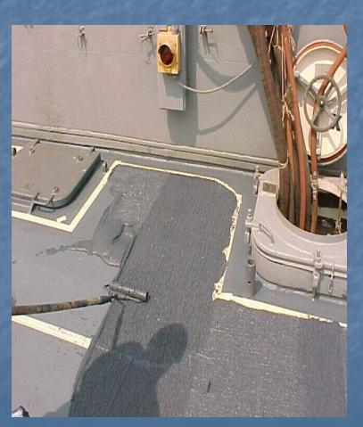
WELDS AND OTHER PROTRUSIONS ARE CROSS ROLLED TO ENSURE THERE ARE NO GAPS OR HOLIDAYS AND TO ENSURE MATERIALS IS PUSHED INTO CONTACT WITH THE SIDES OF THE WELDS ALWAYS KEEP A "WET WORKING PUDDLE" OF FRESH NON-SKID IN FRONT OF THE ROLLER.
